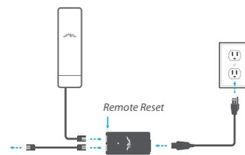
The NanoStationM may also be powered by the Ubiquiti Networks TOUGHSwitch PoE. In addition, any NanoStationM can easily become 48V, 802.3af compliant through use of the Ubiquiti Instant 802.3af Adapter (sold separately).
